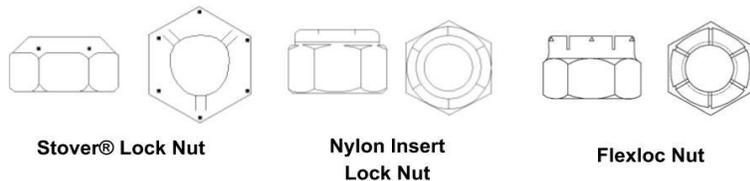
Lock nuts like these are designed to add resistance when installed and generate lots of heat. So avoid them, or install them very slowly. Nylon insert lock nuts paired with stainless steel is a common troublesome issue.
