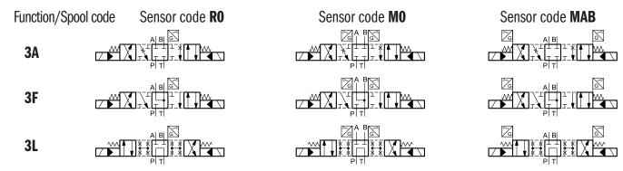
Central position monitored with one positioning sensor De-energized position monitored by two positioning sensor Both external positions monitored by two positioning sensors
