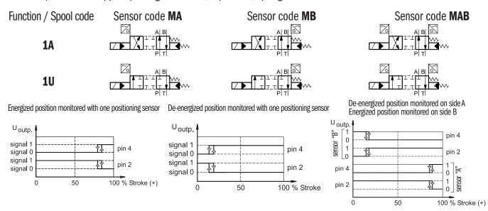
CODE 1 with code R option (A solenoid supplied) - Single solenoid, 2 position, spring offset
