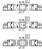
Central position monitored with one positioning sensor
