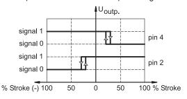
CODE 5 (B solenoid supplied) - Single solenoid, 2 position, spring centered
