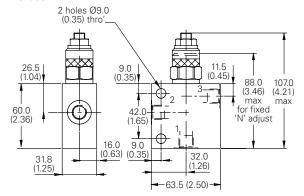
Dual Valve 3/8". 1/2" Ports Basic Code 1CEEB34 Internally Cross Piloted
