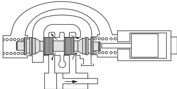
The armature tube area is isolated from the tank port area by the outboard lands on the 4-land spool. Tank port pressure surges do not reach the armature tube to cause failure.
