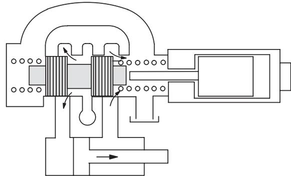
Pressure surges can occur within the armature tube of 2-land wet armature valves due to cylinder port decompression. These surges can easily exceed tube pressure rating and result in premature tube failure.
