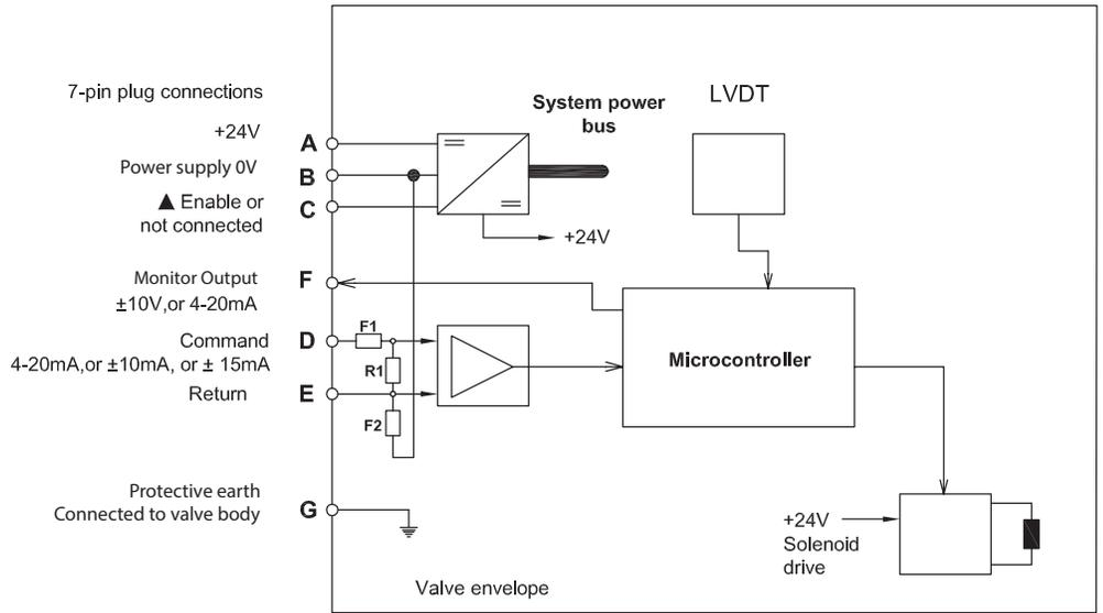
▲ Pin C is used for a valve enable signal with electrical connections Field = H or R
