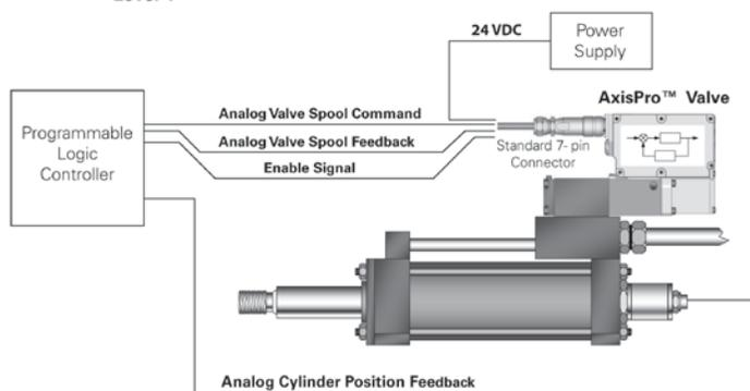
AxisPro level 1 KBH valves, can be used to control machine motions in open loop or closed loop control applications. The valve receives its analog command input on the 7-pin, main, connector from an external axis control device.
