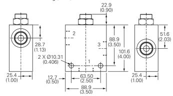
Note: Torque cartridge in aluminum housing to 81-95 Nm (60-70 ft. lbs)
