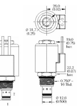
Note: When solenoid valve is ordered as cartridge only, nut is included.
