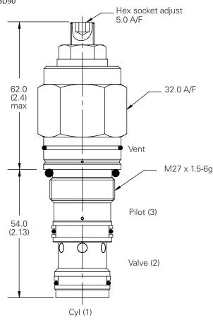
Note: Tightening torque of "F" adjuster locknut - 20 to 25 Nm
