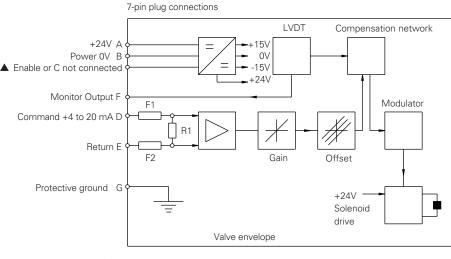
Pin C is used for a valve enable signal with electrical connections PH7.
