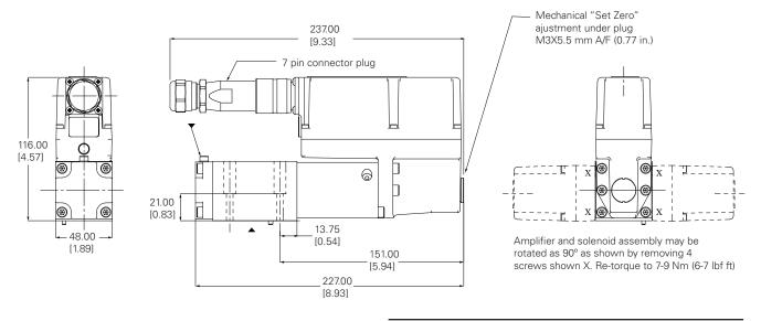
▲ Mounting surface seals supplied. For mounting surface dimensions and subplate options see page 11.
