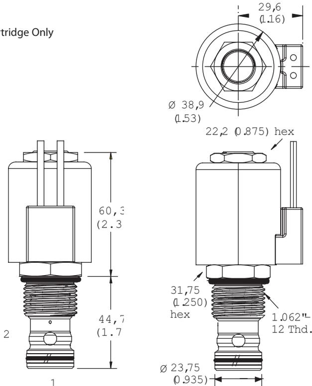
Torque cartridge in housing
