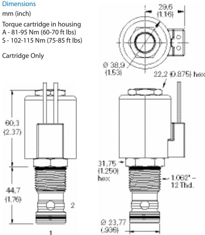
Note: When solenoid valve is ordered as cartridge only, coil nut is included.
