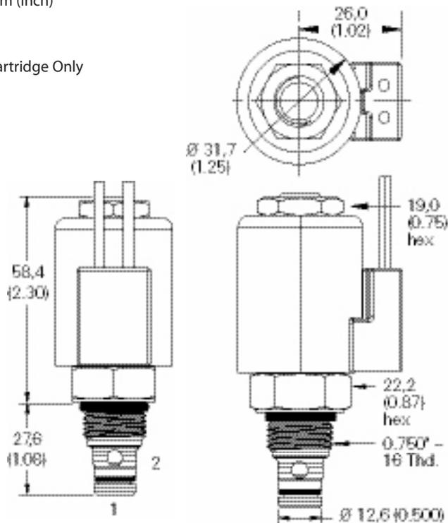
Torque cartridge in steel housing 34-41 Nm (25-30 ft lbs)
